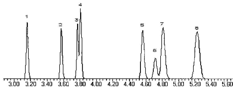
This chromatogram represents a general set of testing conditions chosen for product acceptance. For optimal results in your lab, conditions should be adjusted for your specific instrument, method, and application.
